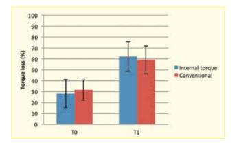
FIG. 1 Percentage of torque loss of conventional and internal torque implants, before and after cyclic loading.
