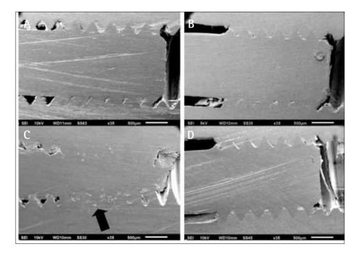
FIG. 2 SEM images of the implant/ abutment/screw assemblies at a 35X magnification. A: Conventional EH before loading; B: Internal torque EH before loading;
