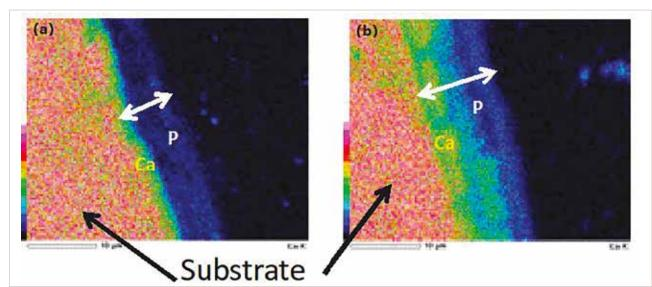
FIG. 5 EDS of the specimen surface (Cross section view) (a) Control group (b) LIPUS group.
