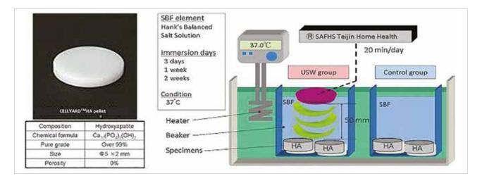
FIG. 1 Diagram of the pulsed ultrasound waving radiation on hydroxyapatite specimens in simulated body fluid (SBF).
