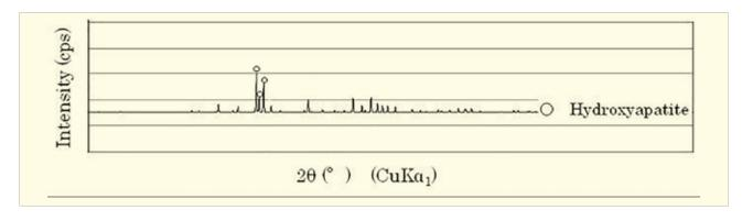
FIG. 6 XRD of the hydroxyapatite surface after soaking in SBF for 2weeks.
