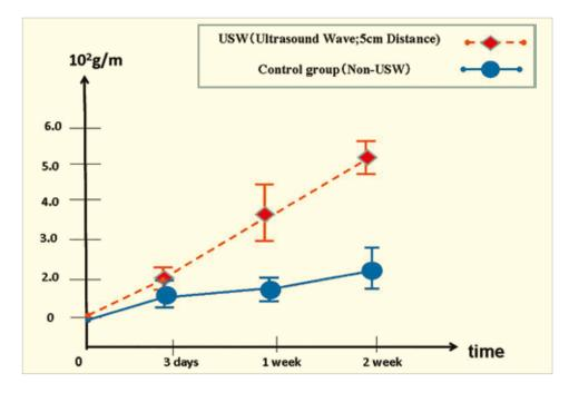
FIG. 7 Soaking time dependence of mass of P/Ca precipitation formation on hydroxyapatite (HA) specimen's surface (radiation distance: 50 mm).
