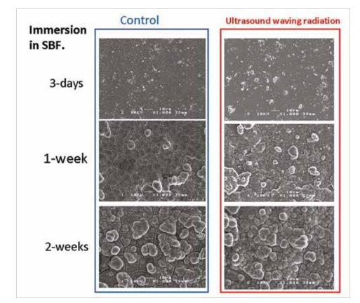
FIG. 4 SEM micrographs of the hydroxyapatite specimen surface after SBF soaking (1000 ×).
