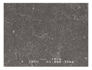
FIG. 3 SEM micrographs o the hydroxyapataite specimens surface before SBF soaking ( $1000 \times$ ).
