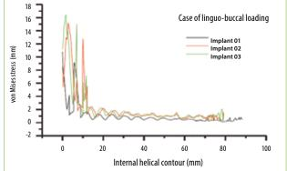
FIG. 7 Variation of the interfacial stress at the bottom of the implant thread depending on the nature of the thread for lateral loading.
