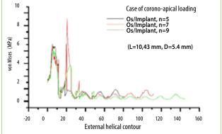
FIG. 9 Variation of interfacial stress outside the implant net depending on the number of nets.
