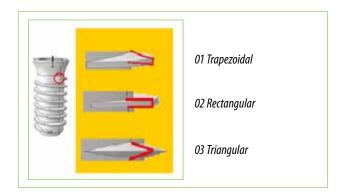
FIG. 1 Implant system components and thread types.
