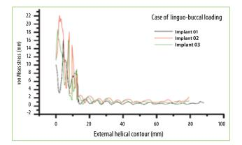
FIG. 6 Interfacial stress variation outside the implant thread depending on the nature of the thread for lateral loading.
