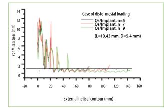
FIG. 11 Variation of the interfacial stress on the outside of the implant net depending on the number of nets.
