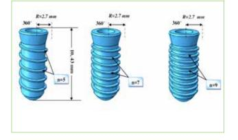
FIG. 8 Geometric model of the dental implant with its dimension.
