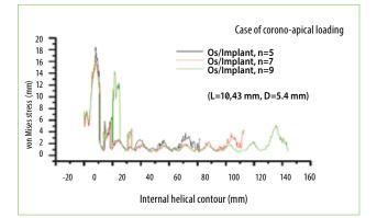
FIG. 10 Variation of interfacial stress outside the implant threads depending on the number of threads.
