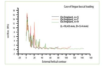
FIG. 13 Variation of the interfacial stress on the outside of the implant net depending on the number of nets.
