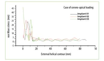
FIG. 2 Variation in interfacial stress outside the implant net depending on the nature of the thread for axial loading.
