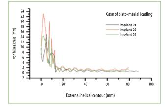
FIG. 4 Variation of the interfacial stress outside the implant thread depending on the nature of the thread for lateral loading.
