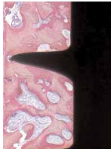
**Fig. 3** No gaps or soft tissues are found at the bone-metal interface. Acid fuchsin and toluidine blue 50X.
