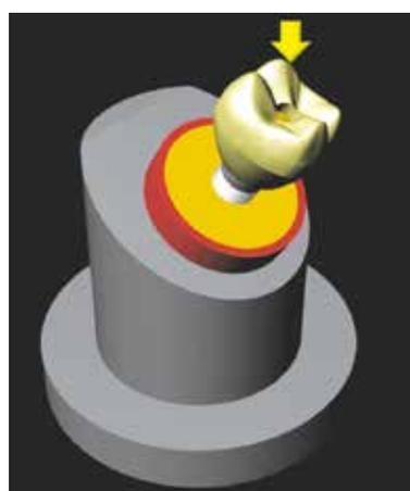
FIG. 2 Final 3D model (ISO 14801) for fixing and applying load (500 N, 30°).
