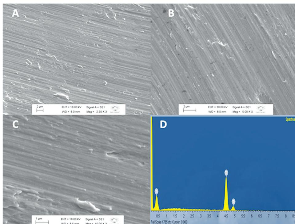
FIG. 1 SEM images at 250x (A), 500x (B) and 1000x (C) and Ti peaks evidenced by the the x-ray energy dispersive spectrometer (EDX) (D) for the MS experimental group.
