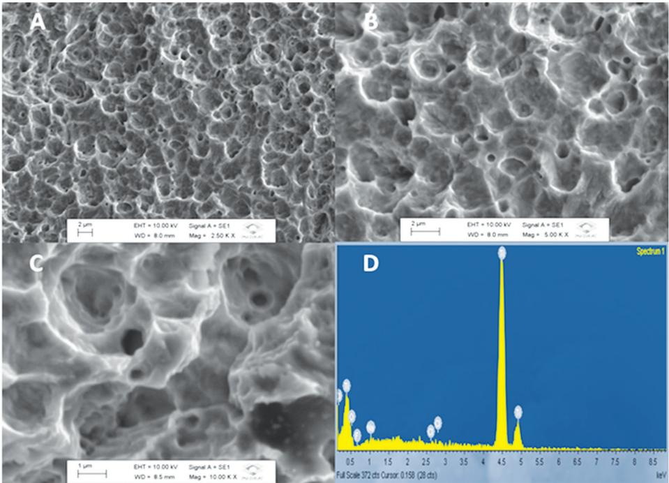
FIG. 2 SEM images at 250x (A), 500x (B) and 1000x (C) and Ti peaks evidenced by the x-ray energy dispersive spectrometer (EDX) (D) for experimental group AFS.
