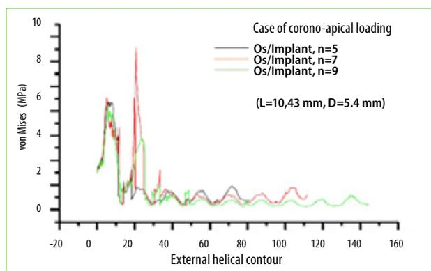
FIG. 9 Variation of interfacial stress outside the implant net depending on the number of nets.
