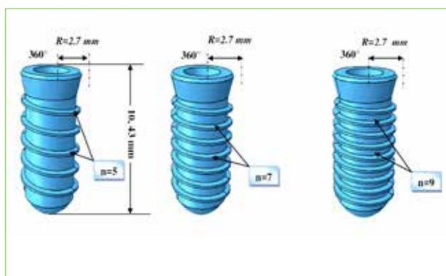
FIG. 8 Geometric model of the dental implant with its dimension.
