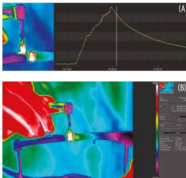
FIG. 1 A: Illustration of the measurement of the generated heat with thermal imaging camera, B: Example for the measurement of the heat generated by S-3.5 drill at 400 rpm
