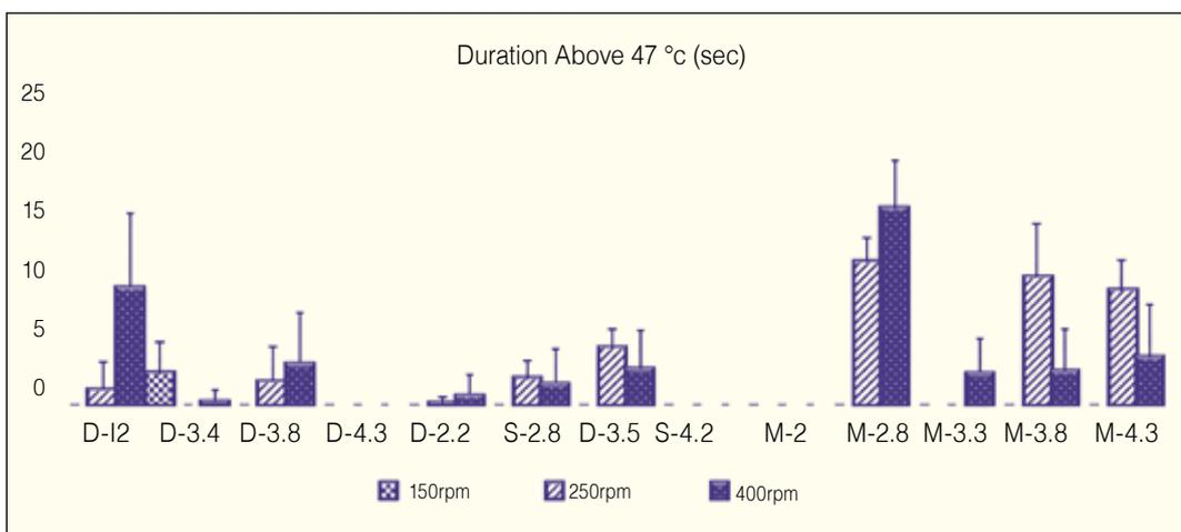
FIG. 4 Comparison of the duration over 47 °C among the drills at different speeds
