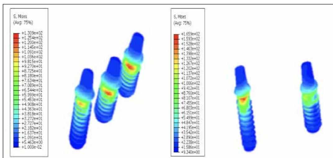
FIG. 6 Contour of von Mises stresses of the implant-abutment part for the dental prosthesis (a) and the dental bridge system (b) at  $t = 5$  sec.
