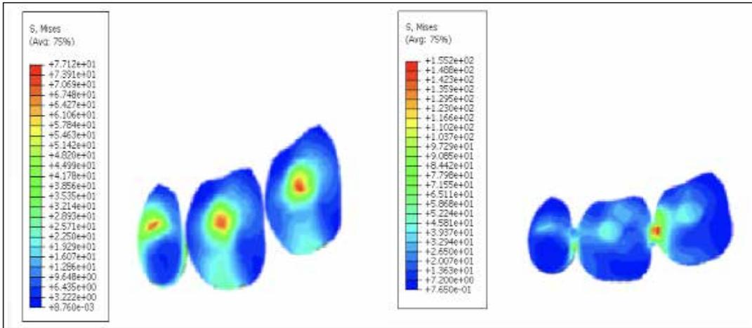
FIG. 7 Contour of the von Mises stresses of the crown gate for the dental prosthesis (a) and the dental bridge system (b) at  $t = 5$  sec.
