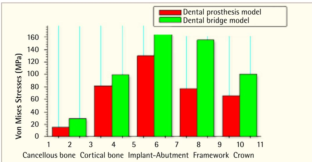
FIG. 9 Histogram of the maximum von Mises stress of the two dental structures.
