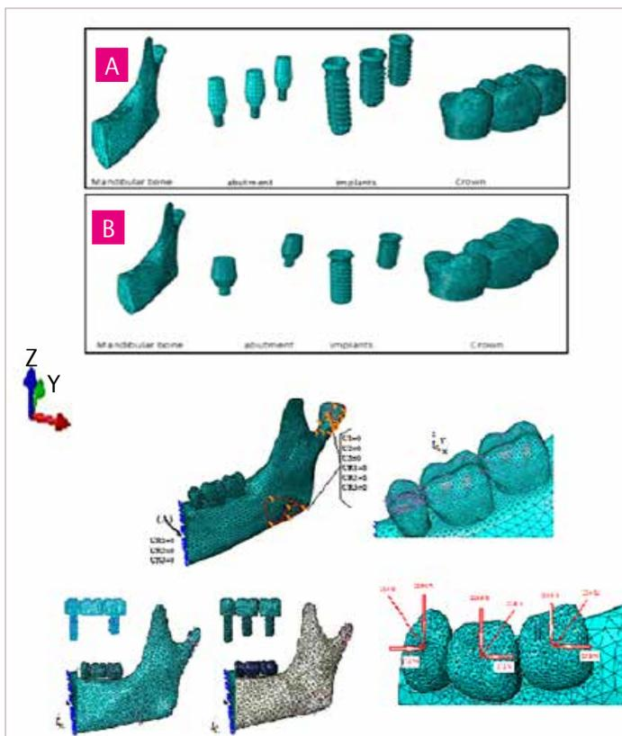
FIG. 4 Mesh using linear tetrahedral elements for a dental prosthesis (a) and a dental bridge system (b).
