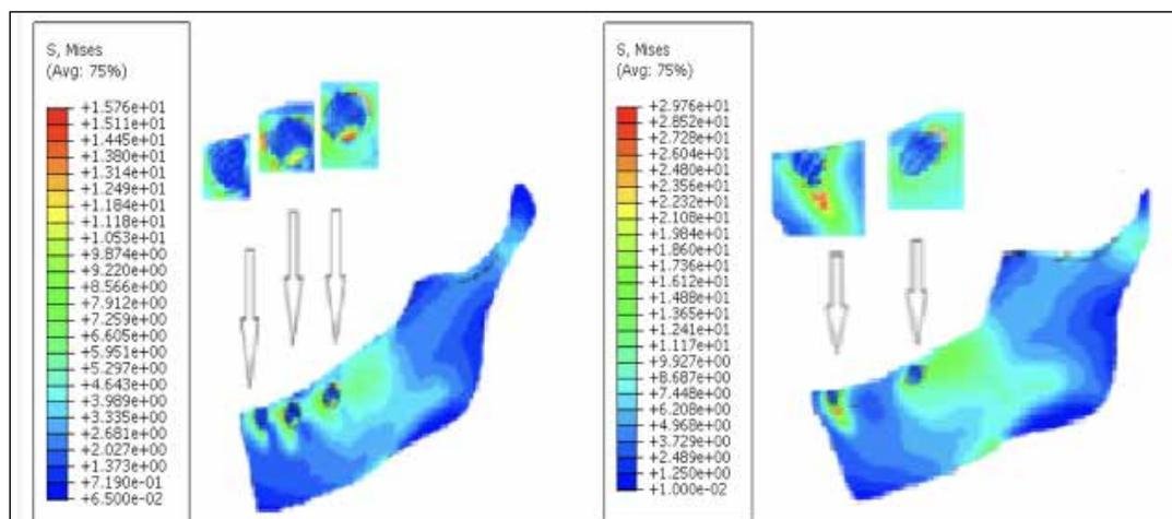
FIG. 5 Contour of von Mises stresses of cancellous bone for the dental prosthesis (a) and the dental bridge system (b) at  $t = 5$  sec.
