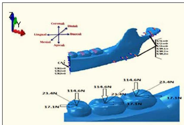
FIG. 2 Boundary conditions: zero displacement, corono-apical, linguo-buccal and disto-mesial loads (12).
