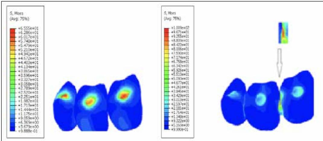
FIG. 8 Contour of the von Mises stresses of the crown for the dental prosthesis (a) and the dental bridge system (b) at  $t = 5$  sec.
