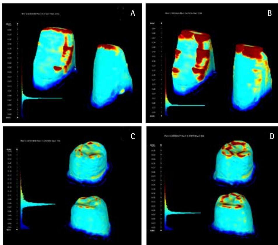
**FIG. 6** Example colourmaps of measurements from the intaglio surface of the designed crowns, two viewing angles of the same design are shown.
