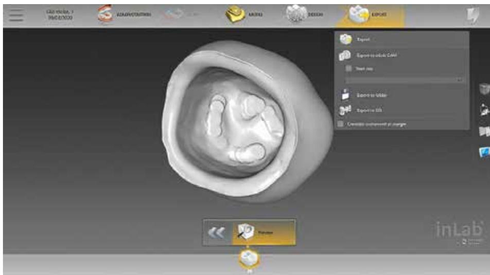
FIG. 2 Bur marks on the internal surface of crown design displayed by inLab SW.
