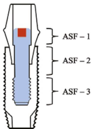
FIG. 3 Parts of the abutment screw.
