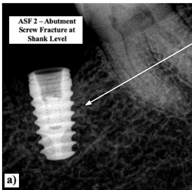
FIG. 5 Example of abutment screw fracture at shank level.
