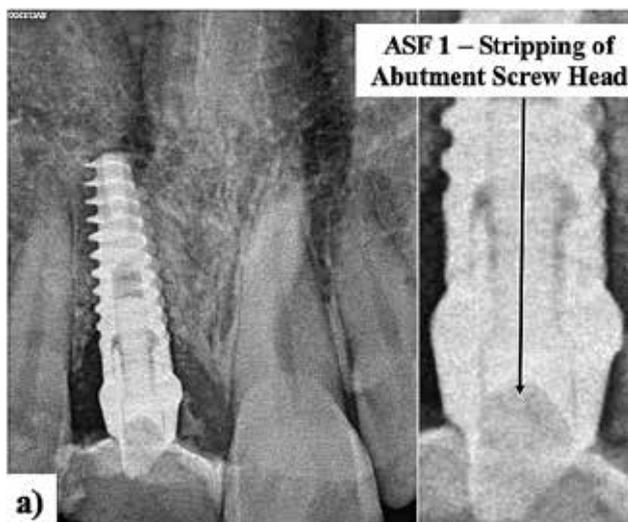
FIG. 4 Example of abutment screw fracture at head level.
