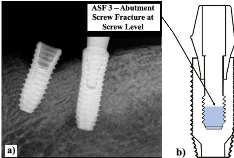
**FIG. 6** Example of abutment screw fracture at screw level.
