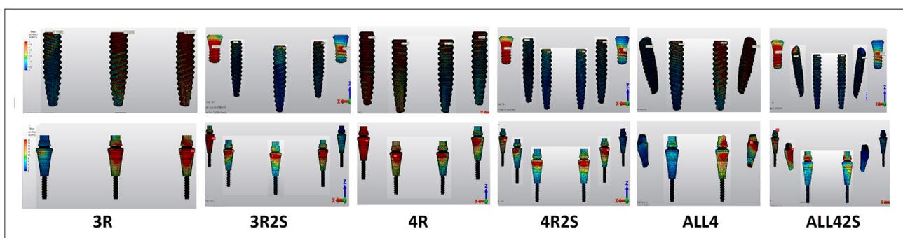
FIG. 8. Stress values and distributions in the multiunit abutments against canine and molar forces
