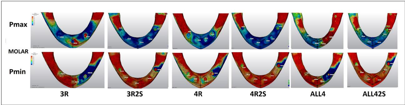
FIG. 5. Stress values and distributions in the cortical bone against molar forces
