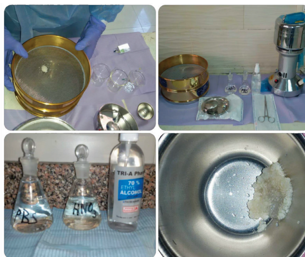
FIG. 3 Sieving for particle size selection followed by chemical processing to obtain the graft in its final form
