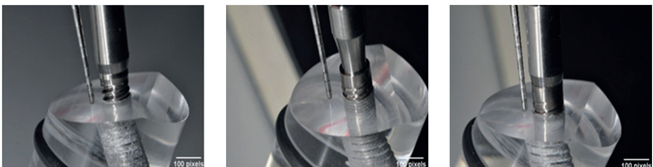
Fig. 1 Stub equipped for implant fixation and the distance of 3 mm from the platform to the implant's exposed location to simulate a critical case of bone resorption.
